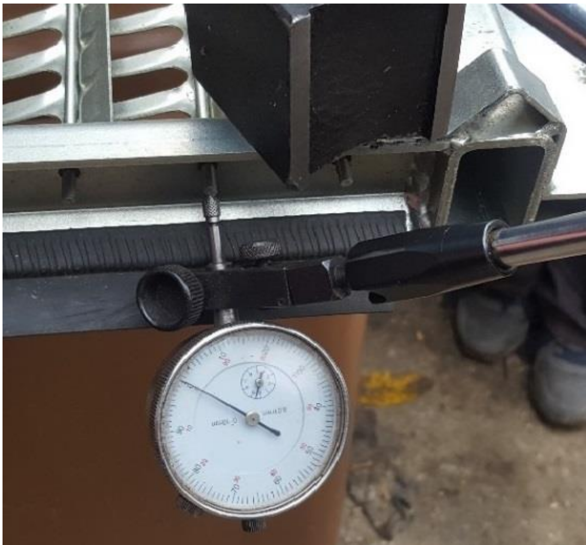
Photo 7 Zero sensor in the lower position of the lamella rotation axis.
