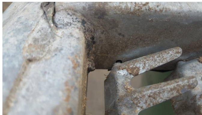
Photo 6 Excessive clearance between the axis of rotation of the lamellas and the sieve frame in the sieve removed from the combine harvester.
