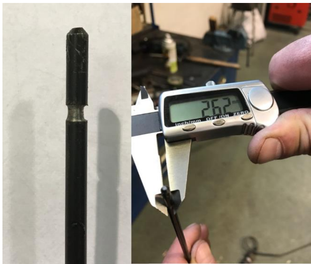
Photo 4 The diameter of the axis of rotation of the lamella after removal from the frame (nominal diameter 3.8 mm).
