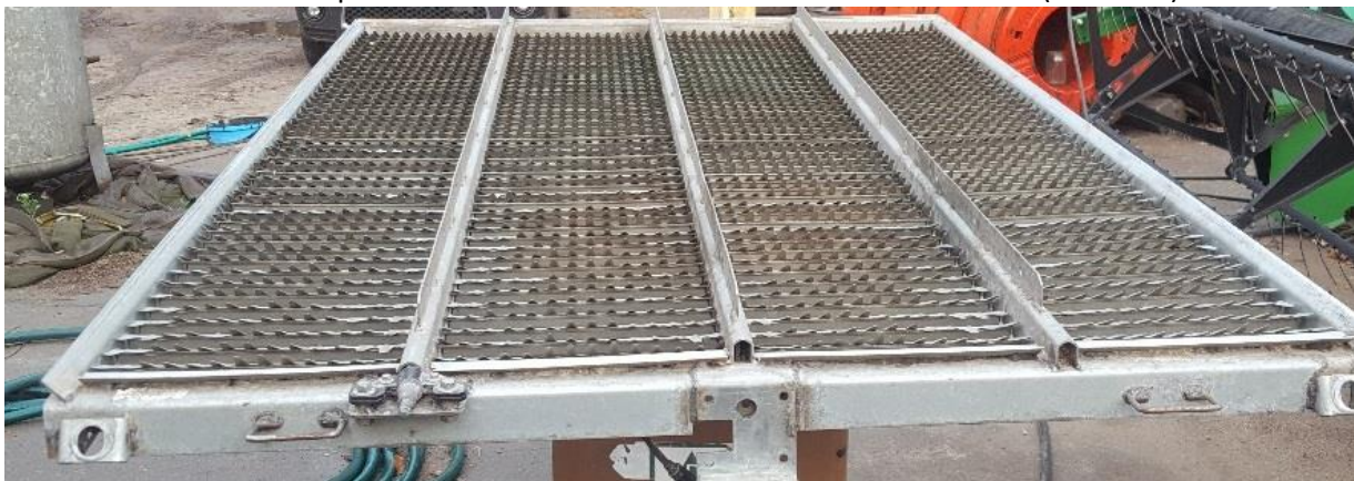
Photo 10 Sieve with CZ3 lamella with visible deformation of lamellas after 140 hours of operation.
