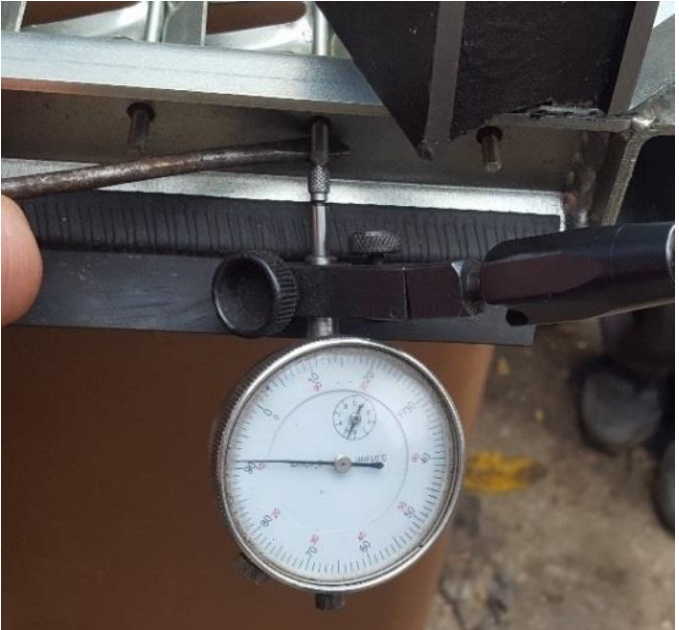
Photo 8 The sensor indicates a deviation of 0.09 mm. in the upper position of the axis of rotation of the lamellas.
