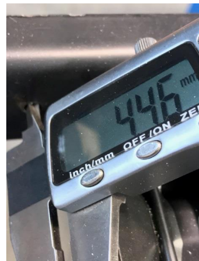
Photo 5 Diameter of the hole in the sieve frame (nominal diameter d = 3.9 mm).
