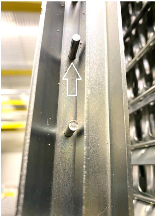
Photo 1 – The method of placing the lamella rotation axes in the calibrated hole
