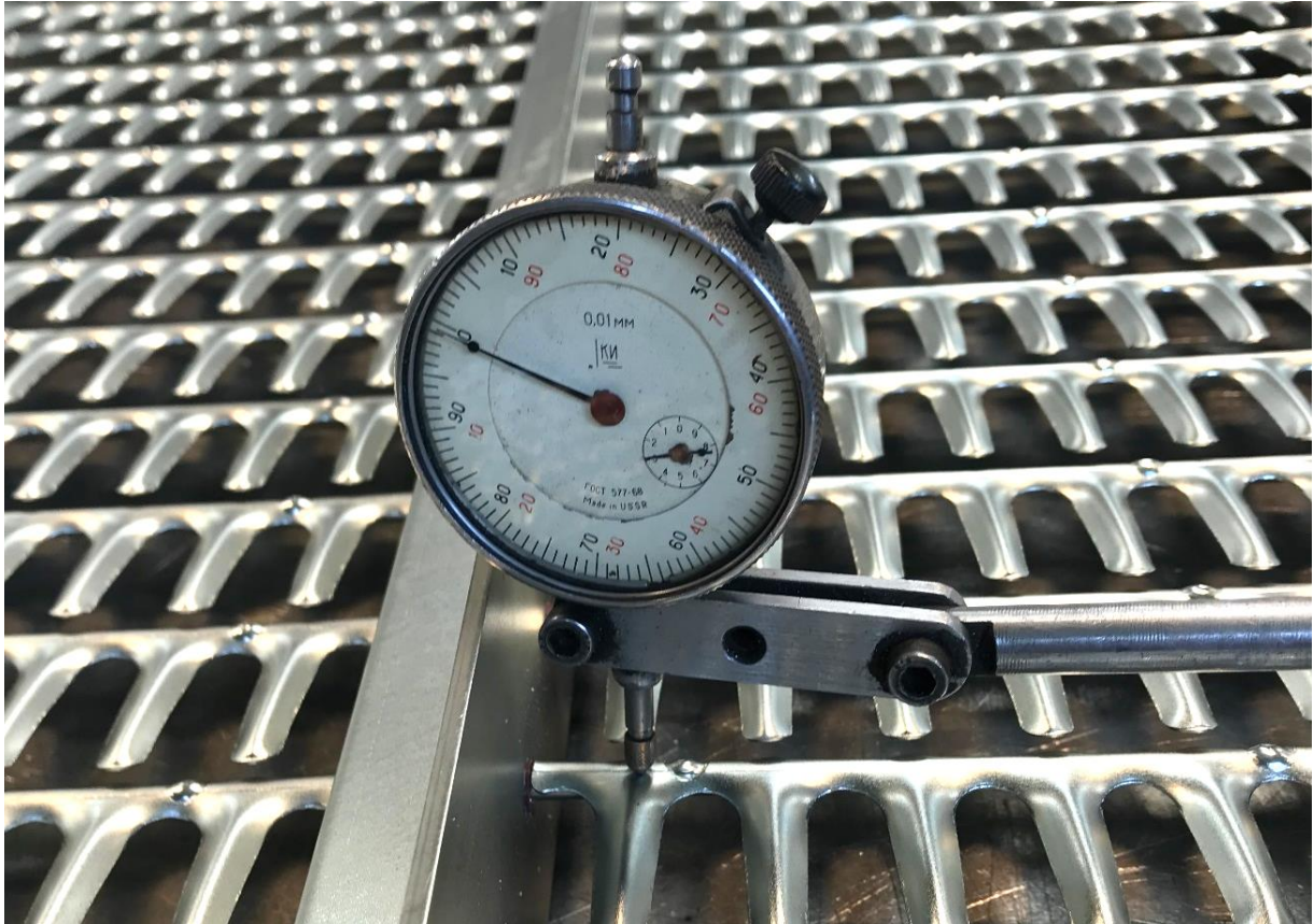
Photo 3- The method of measuring the clearance with a time sensor
